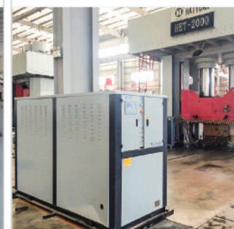
■ The tmperature control of large press
